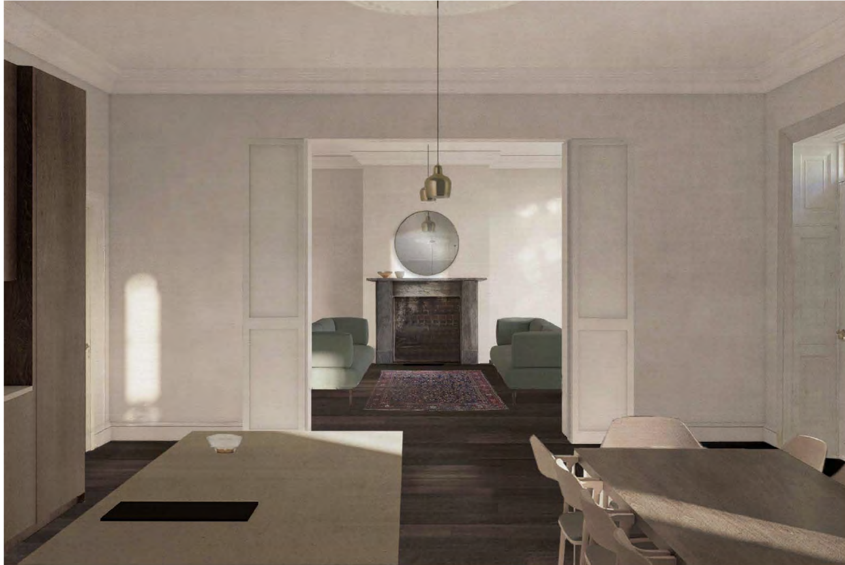
The blocked up fire place in the ground floor living room G6 will be opened up and provided with a sympathetic surround and mantelpiece.
